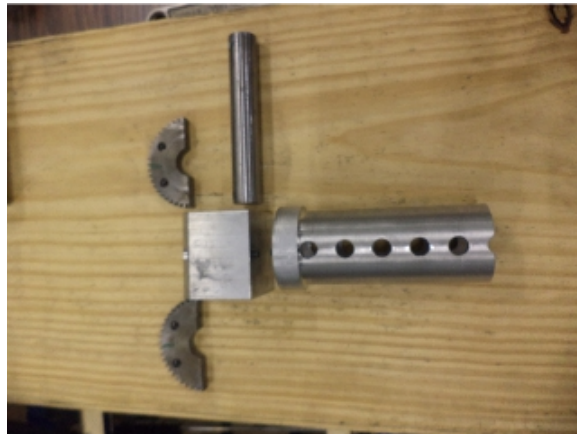
Figure A.2: Knee Assembly Dismantled
